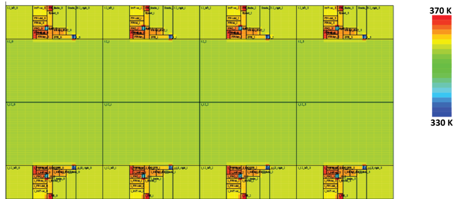
Figure 6.2 Steady state temperature profile for an oct-core processor. The floorplan is Generated by Mirroring and Replicating the Single Core floorplan
